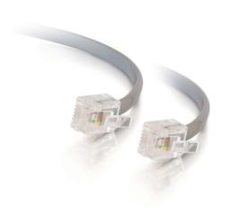
Constructed from heavy duty 28 AWG silver satin wire, this cable has gold-plated connectors for clearer communication. Its 4-wire construction handles dual phone lines while the heavy duty PVC jacket protects the cable's integrity.
