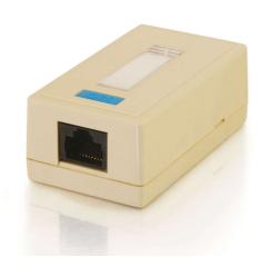
Ideal for surface mount applications, especially in confined spaces. Mount for either side or base entry of cables. Boxes come with mounting screws and adhesive tape, and a cable tie for strain relief. The snap-on cover enables easy closure or access for quick installation. Each box includes a write-on label with holder for easy designation of different system or station. Contacts are phosphor bronze plated with 50 inch hard gold.
